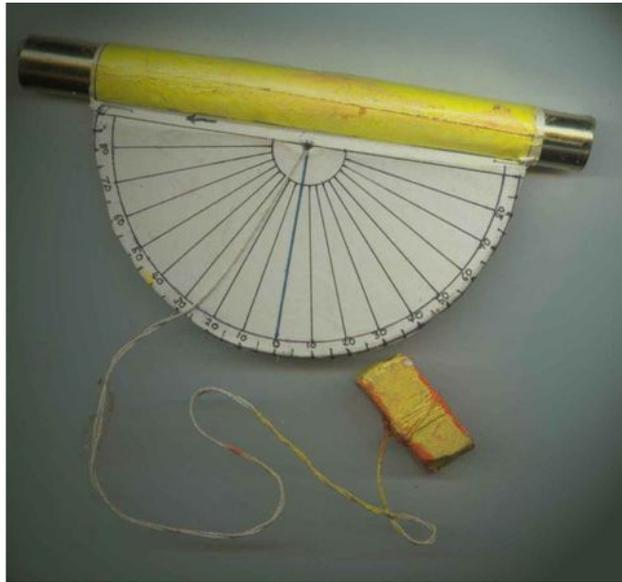
*An inclinometer. Inclinometers can be used to measure angles of inclination and so can be used to determine the height of an object.*
