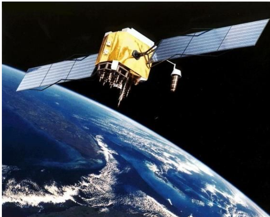
Figure 1: An artist's depiction of a GPS satellite orbiting the Earth. There are at least 24 GPS satellites operational at any one time. GPS uses an application of trigonometry, known as triangulation, to determine one's position. The accuracy of GPS is to within 15 metres.
